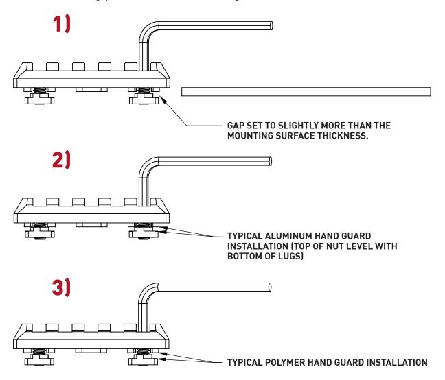
Some Magpul accessories may arrive preset to the condition shown in the illustration for easy installation on aluminum hand guards. Remember to loosen the nuts a bit for polymer installation.
